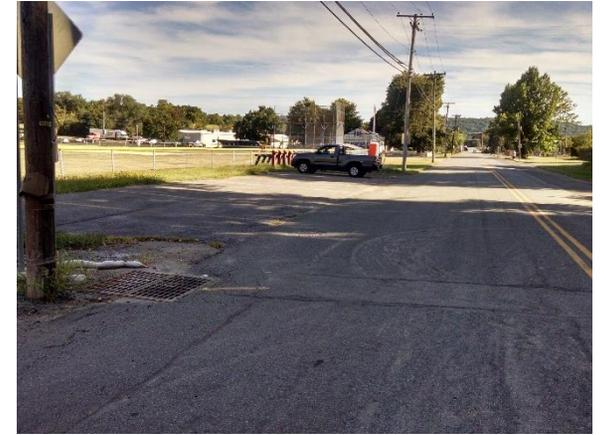
Parking spots to the north of the field can be replaced with porous asphalt to capture and infiltrate stormwater. Installing a rain garden adjacent to the road can capture, treat, and infiltrate road runoff. A preliminary soil assessment suggests that more soil testing would be required before determining the soil's suitability for green infrastructure.
