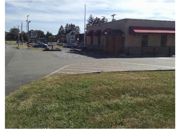
Parking spots to the east and west of the building can be replaced with porous asphalt to capture and infiltrate stormwater. A preliminary soil assessment suggests that the soils have suitable drainage characteristics for green infrastructure.
