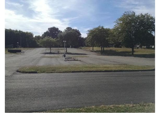
Parking spots in the middle of the parking lot and the playground in the northeastern corner can be replaced with porous asphalt to capture and infiltrate stormwater. Installing bioretention systems in the parking lot and adjacent to the road can capture, treat, and infiltrate runoff. A preliminary soil assessment suggests that more soil testing would be required before determining the soil's suitability for green infrastructure.
