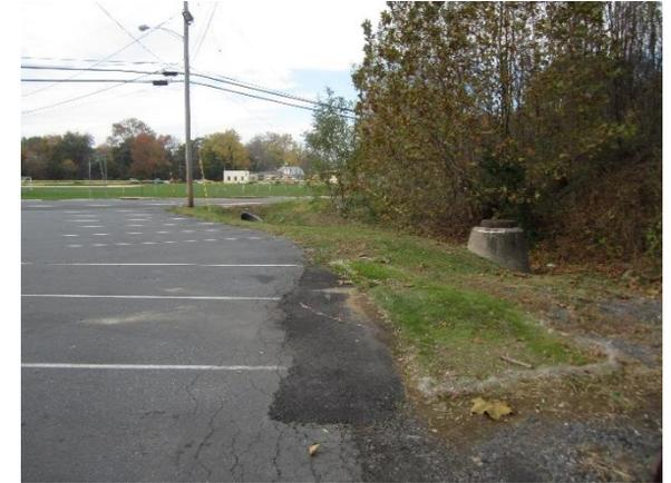
Installing a rain garden adjacent to the building can capture, treat, and infiltrate roof runoff, and another rain garden can be installed north of parking spaces to infiltrate parking lot runoff. A preliminary soil assessment suggests that the soils have suitable drainage characteristics for green infrastructure.
